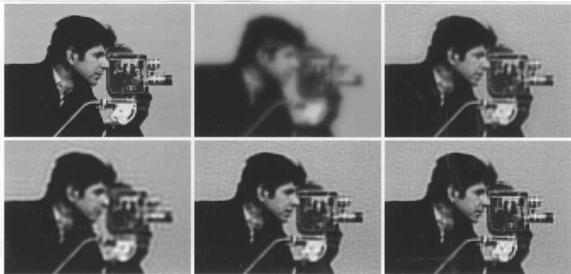
Figure 8.7–26. subband EM restoration of cameraman at \text{BSNR} = 40 \text{ dB} , \begin{bmatrix} a & b & c \\ d & e & f \end{bmatrix} a -original, b -blurred, c , fullband restored, d - LL subband restored, e - subband (LSI), f - subband (LSV) (from [??] © 1994 IEEE)
