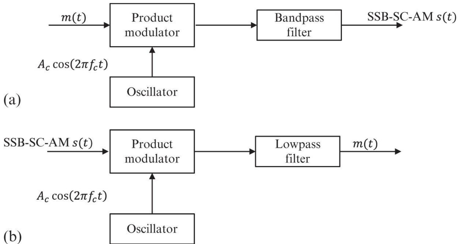
**Figure A.12** SSB-SC AM: (a) modulator and (b) coherent demodulator.
