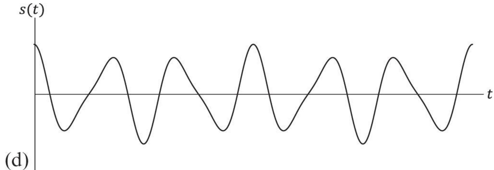
**Figure A.15d** Signals in the time domain: (a) modulating signal, (b) carrier wave, (c) SSB-SC (LSB), (d) VSB-SC (LSB), (e) DSB-SC, (f) VSB-SC (USB), (g) SSB-SC (USB), (h) SSB-PC (LSB), (i) VSB-PC (LSB), (j) DSB-PC, (k) VSB-PC (USB), and (l) SSB-PC (USB).
