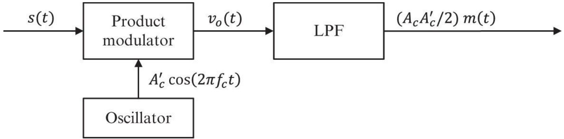
**Figure A.10** Coherent detection of DSB-SC-AM signal.
