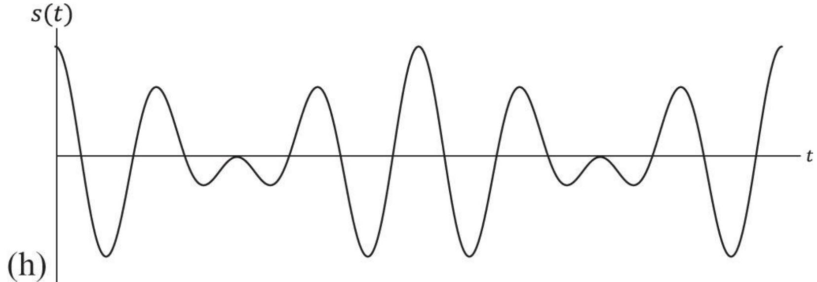
**Figure A.15h** Signals in the time domain: (a) modulating signal, (b) carrier wave, (c) SSB-SC (LSB), (d) VSB-SC (LSB), (e) DSB-SC, (f) VSB-SC (USB), (g) SSB-SC (USB), (h) SSB-PC (LSB), (i) VSB-PC (LSB), (j) DSB-PC, (k) VSB-PC (USB), and (l) SSB-PC (USB).
