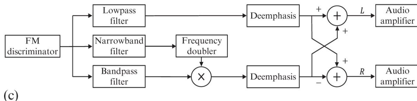
**Figure A.25** FM stereo broadcasting: (a) FM stereo transmitter, (b) spectrum of FM stereo signal, and (c) FM stereo receiver.
