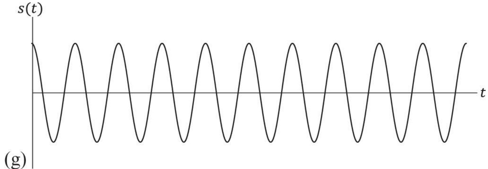
**Figure A.15g** Signals in the time domain: (a) modulating signal, (b) carrier wave, (c) SSB-SC (LSB), (d) VSB-SC (LSB), (e) DSB-SC, (f) VSB-SC (USB), (g) SSB-SC (USB), (h) SSB-PC (LSB), (i) VSB-PC (LSB), (j) DSB-PC, (k) VSB-PC (USB), and (l) SSB-PC (USB).
