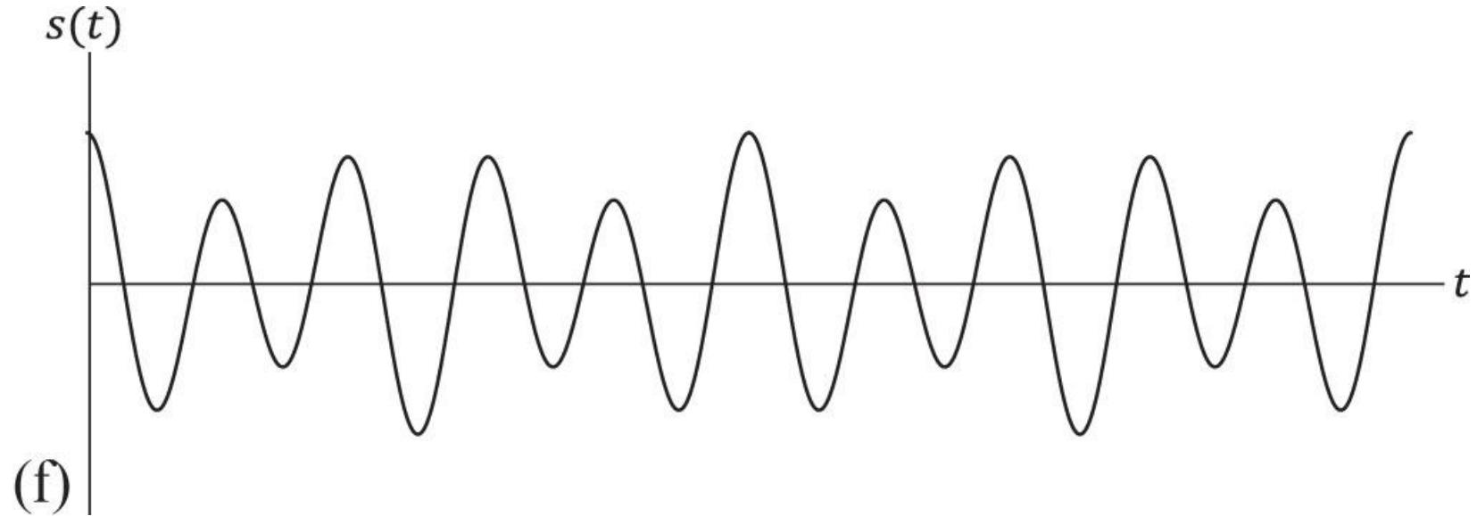
**Figure A.15f** Signals in the time domain: (a) modulating signal, (b) carrier wave, (c) SSB-SC (LSB), (d) VSB-SC (LSB), (e) DSB-SC, (f) VSB-SC (USB), (g) SSB-SC (USB), (h) SSB-PC (LSB), (i) VSB-PC (LSB), (j) DSB-PC, (k) VSB-PC (USB), and (l) SSB-PC (USB).
