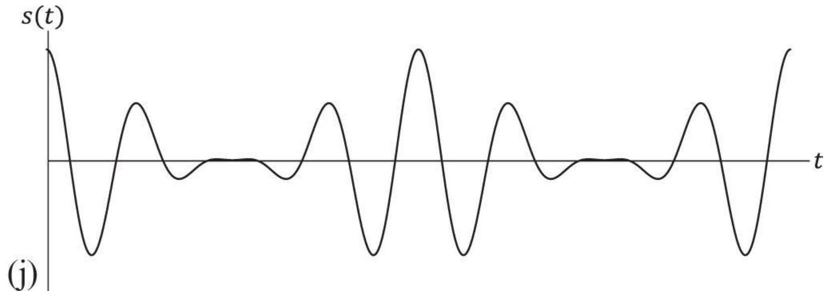
**Figure A.15j** Signals in the time domain: (a) modulating signal, (b) carrier wave, (c) SSB-SC (LSB), (d) VSB-SC (LSB), (e) DSB-SC, (f) VSB-SC (USB), (g) SSB-SC (USB), (h) SSB-PC (LSB), (i) VSB-PC (LSB), (j) DSB-PC, (k) VSB-PC (USB), and (l) SSB-PC (USB).
