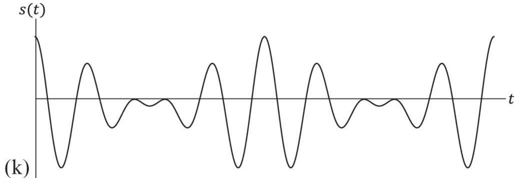
**Figure A.15k** Signals in the time domain: (a) modulating signal, (b) carrier wave, (c) SSB-SC (LSB), (d) VSB-SC (LSB), (e) DSB-SC, (f) VSB-SC (USB), (g) SSB-SC (USB), (h) SSB-PC (LSB), (i) VSB-PC (LSB), (j) DSB-PC, (k) VSB-PC (USB), and (l) SSB-PC (USB).
