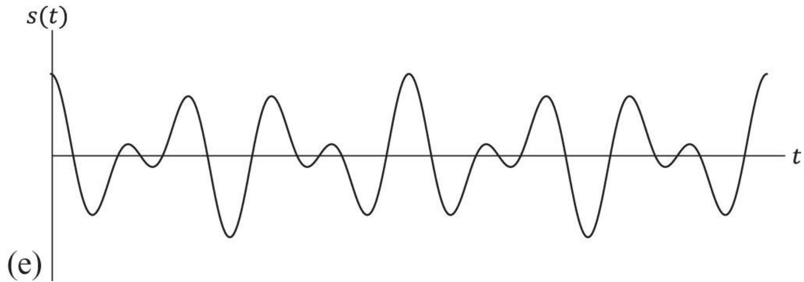
**Figure A.15e** Signals in the time domain: (a) modulating signal, (b) carrier wave, (c) SSB-SC (LSB), (d) VSB-SC (LSB), (e) DSB-SC, (f) VSB-SC (USB), (g) SSB-SC (USB), (h) SSB-PC (LSB), (i) VSB-PC (LSB), (j) DSB-PC, (k) VSB-PC (USB), and (l) SSB-PC (USB).
