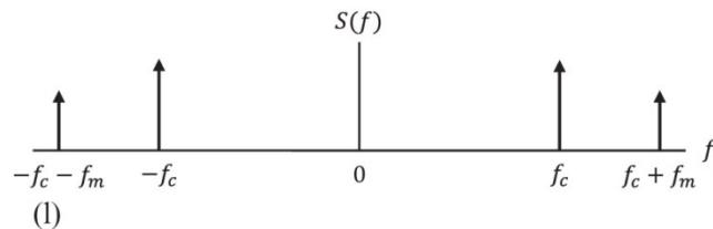
**Figure A.1h-l** Signals in the frequency domain: (a) modulating signal, (b) carrier wave, (c) SSB-SC (LSB), (d) VSB-SC (LSB), (e) DSB-SC, (f) VSB-SC (USB), (g) SSB-SC (USB), (h) SSB-PC (LSB), (i) VSB-PC (LSB), (j) DSB-PC, (k) VSB-PC (USB), and (l) SSBPC (USB).
