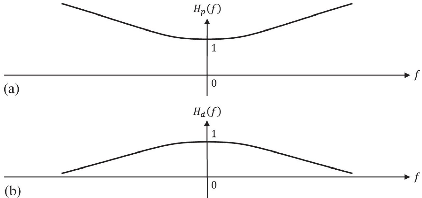
**Figure A.21** Pre-emphasis and de-emphasis filters characteristics.
