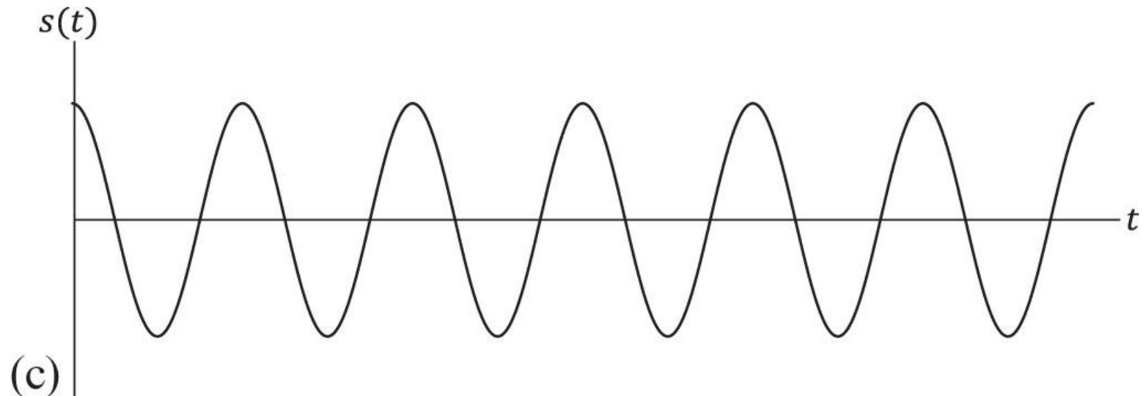
**Figure A.15c** Signals in the time domain: (a) modulating signal, (b) carrier wave, (c) SSB-SC (LSB), (d) VSB-SC (LSB), (e) DSB-SC, (f) VSB-SC (USB), (g) SSB-SC (USB), (h) SSB-PC (LSB), (i) VSB-PC (LSB), (j) DSB-PC, (k) VSB-PC (USB), and (l) SSB-PC (USB).
