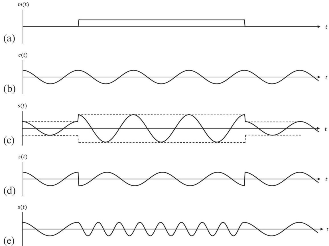
**Figure A.2** CW modulation for a rectangular pulse: (a) rectangular modulating signal, (b) carrier wave, (c) amplitude modulated signal, (d) phase modulated signal, and (e) frequency modulated signal.
