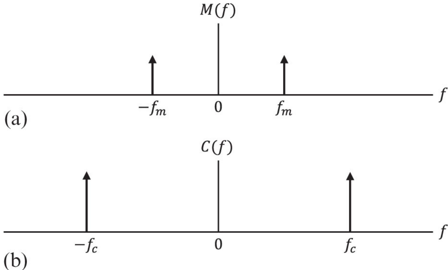
**Figure A.16ab** Signals in the frequency domain: (a) modulating signal, (b) carrier wave, (c) SSB-SC (LSB), (d) VSB-SC (LSB), (e) DSB-SC, (f) VSB-SC (USB), (g) SSB-SC (USB), (h) SSB-PC (LSB), (i) VSB-PC (LSB), (j) DSB-PC, (k) VSB-PC (USB), and (l) SSBPC (USB).
