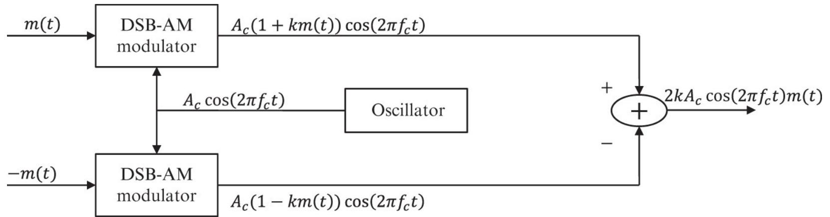
**Figure A.9** Balanced modulator for DBS-SC AM.
