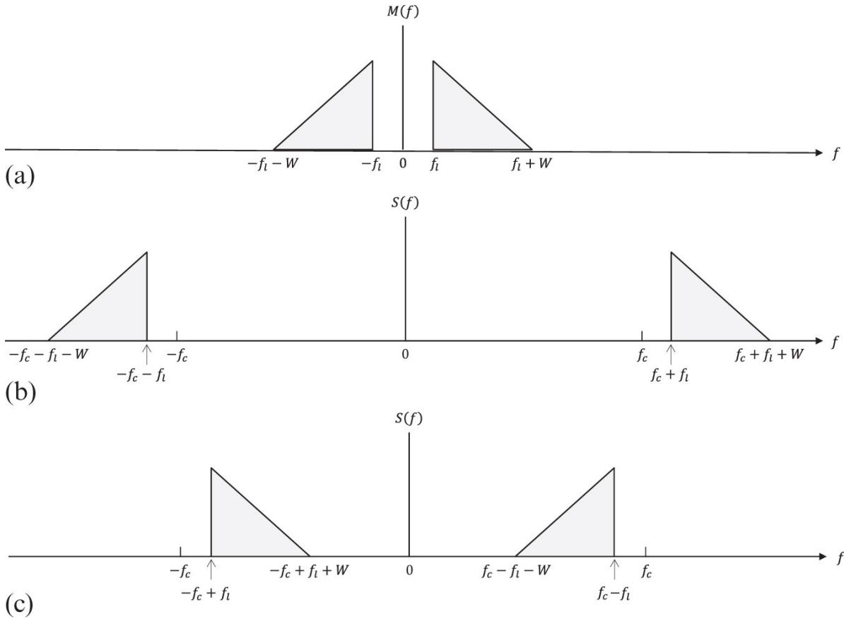
**Figure A.11** Spectrum: (a) modulating signal, (b) SSB-SC AM (USB), and (c) SSB-SC AM (LSB).
