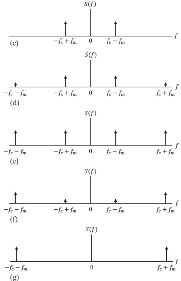
**Figure A.1a-g** Signals in the frequency domain: (a) modulating signal, (b) carrier wave, (c) SSB-SC (LSB), (d) VSB-SC (LSB), (e) DSB-SC, (f) VSB-SC (USB), (g) SSB-SC (USB), (h) SSB-PC (LSB), (i) VSB-PC (LSB), (j) DSB-PC, (k) VSB-PC (USB), and (l) SSBPC (USB).
