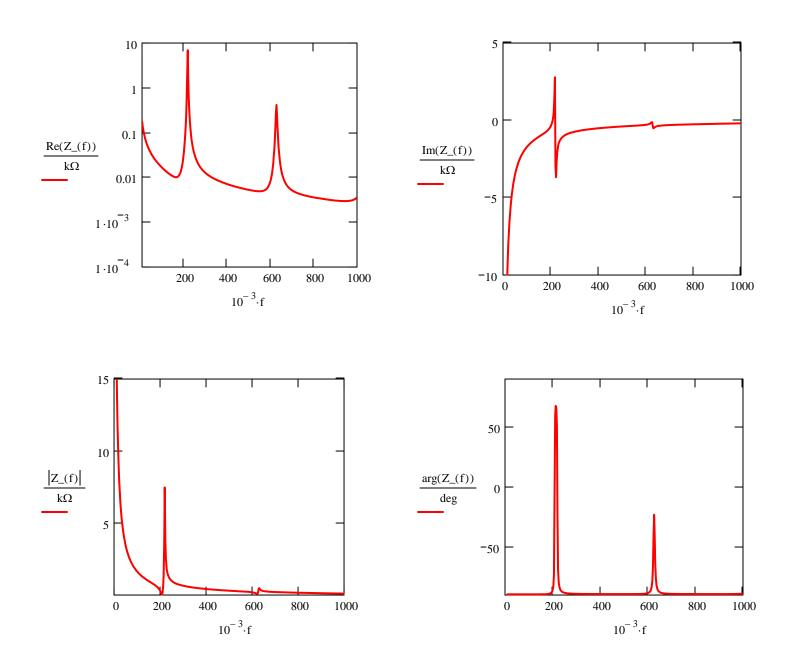
**Problem 2**: Consider a circular PWAS transducer with diameter 2a = 7 mm, thickness  $t_a = 0.2$  mm, and piezoelectric material properties as given in Table 7.1. Assume internal damping ratio  $\eta = 1\%$  and electric loss factor  $\delta = 1\%$ .
