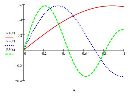
(iv) and (v): the calculation of admittance Y and impedance Z is done in MATLAB because MathCad cannot handle Bessel functions with complex arguments
