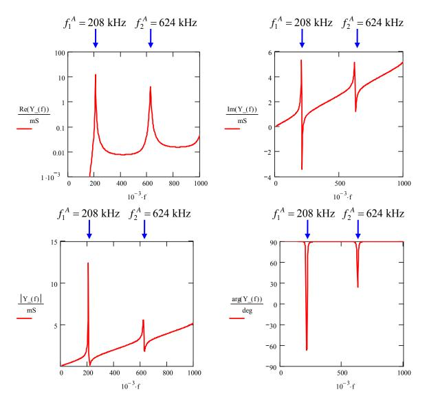
The chart of admittance vs. frequency shows peaks at  $f_1^Y = 208 \text{ kHz}$ ,  $f_2^Y = 624 \text{ kHz}$ . These are antisymmetric frequencies  $f_1^A = 208 \text{ kHz}$ ,  $f_2^A = 624 \text{ kHz}$ , at which the PWAS resonates. As the PWAS passes through these frequencies, its admittance goes through a maximum and takes up a lot of electrical power from the power supply and converts it into mechanical power needed to maintain the PWAS in a state of resonant vibration.
