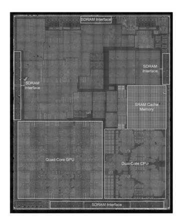
**FIGURE 1.1** The processor integrated circuit inside the Apple A8 chip package. It has two ARM processor cores, four PowerVR G6450 cores, four DRAM interfaces (connections to off-chip memory), an LCD interface, a camera interface, and a USB interface. (*Photo from ChipWorks.*)
