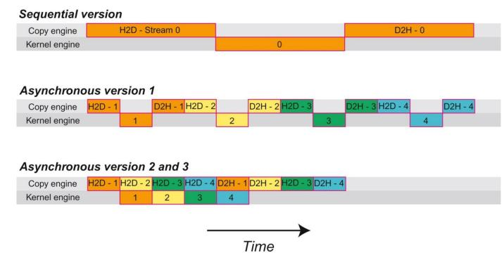
**FIGURE C.1:** Data transfer and kernel execution timing for the sequential and asynchronous versions when there is only one copy engine.
