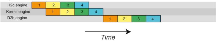
**FIGURE C.2**: Data transfer and kernel execution timing for the sequential and asynchronous versions when there are two copy engines.
