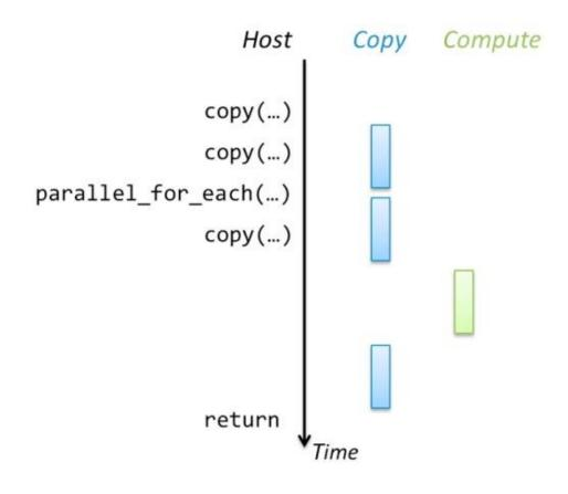
FIGURE D.5: Concurrent host/accelerator execution.
