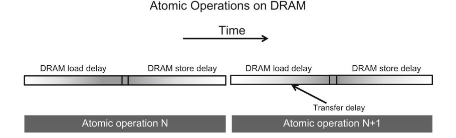
**FIGURE 9.9:** Throughput of atomic operation is determined by the memory access latency.
