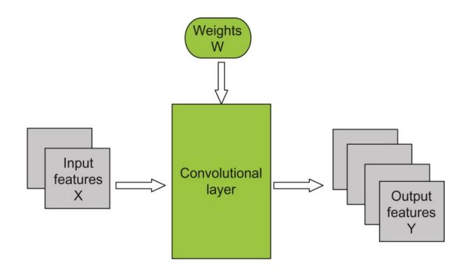
**FIGURE 16.3:** Overview of the forward propagation path of a convolution layer.
