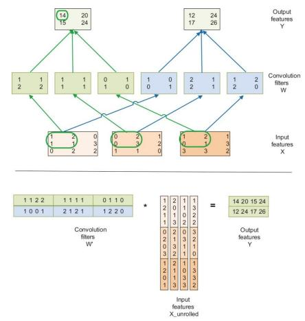
FIGURE 16.14: Reduction of a convolutional layer to GEMM.
