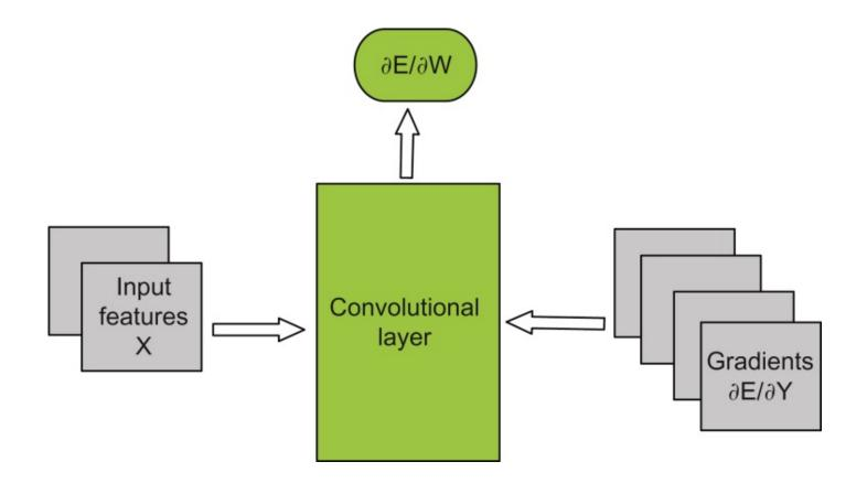
**FIGURE 16.7:** Convolutional layer: Backpropagation of  $\partial E/\partial w$ .
