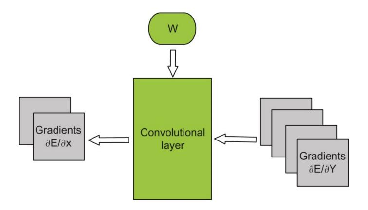
**FIGURE 16.6:** Convolutional layer: Backpropagation of  $\partial E/\partial X$ .
