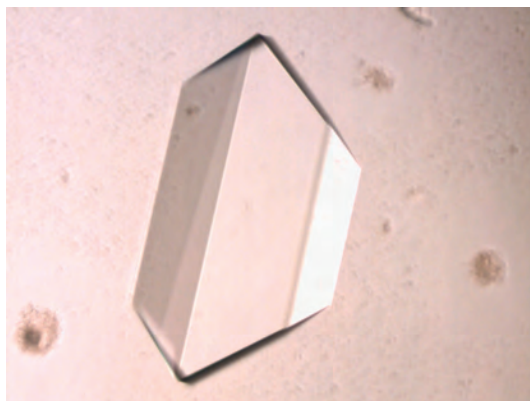
Figure 1 A crystal of yeast inorganic pyrophosphatase grown by temperature-controlled batch crystallization. 23 The longest dimension of the crystal is \sim 700\ \mu\text{m} .
