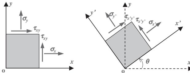
**Figure 2.7** Stress components before and after transformation.
