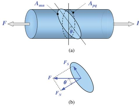
**Figure 2.3** (a) Tensile force applied on a bar, (b) Projected forces parallel and normal to surface  $m-n$ .
