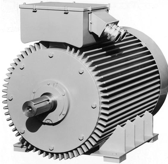
Plate 1.2 *Steel frame cage induction motor, 150 kW (201 h.p.), 1485 rev/min. The active parts are totally enclosed, and cooling is provided by means of an internal fan which circulates cooling air round the interior of the motor through the hollow ribs, and an external fan which blows air over the case. (Photograph by courtesy of Brook Crompton.)*
