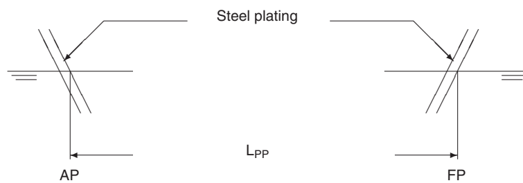
Figure 1.2 How to measure the length between perpendiculars
