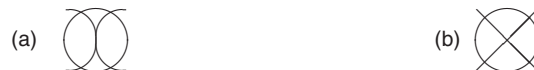
Figure 1.5 (a) Midships symbol in English literature, (b) Midships symbol in German literature
