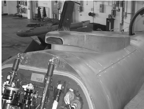
Figure 1.62 Secondary heat exchanger inlet (courtesy of RAF Coltishall)
