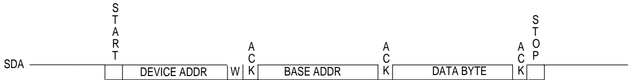
Figure 16-126. Byte Write to Device with Internal Addresses
