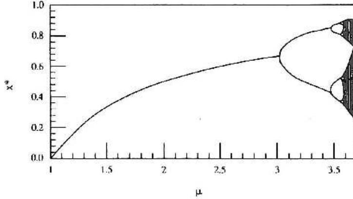
Figure 33.3: Bifurcation plot for the logistic map: Fixed points  $x^*$  versus  $\mu$ .
