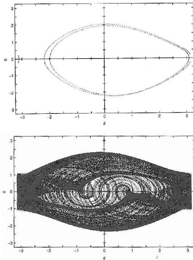
Figure 33.5: 2-D phase-space projections of (a) nonchaotic and (b) chaotic behavior. (From Baker and Gollub, *Chaotic Dynamics*, 2d ed.; used with permission of the copyright holder, Cambridge University Press.)
