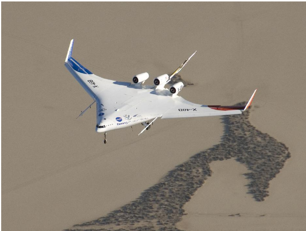
Figure C5-12: In early 2010, a joint NASA/Boeing team completed the first phase of flight tests of the unique X-48B Blended Wing Body aircraft at NASA's Dryden Flight Research Center on Edwards Air Force Base, California. (NASA photo by Tony Landis)
