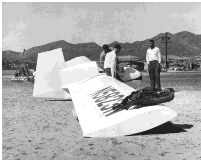
Figure C5-15: The Marske XM-1C flying plank, boasting its Fauvel 14% airfoils. (photo courtesy of Jim Marske).
