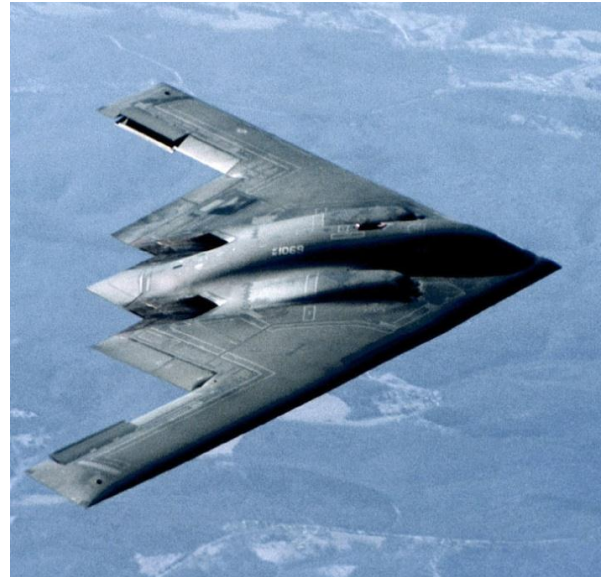
Figure C5-10: Clamshell ailerons on the B-2 Spirit stay open to generate directional stability. (Photo by the Official Web Site of the U.S. Air Force) 10
