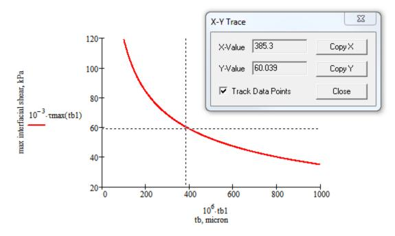
The target shear stress value is half of the value found in item (b) above, i.e.,  $\tau_{\text{max}}^{(b)}/2 \approx 60$  kPa. As shown in the above plot, the approximate value of  $t_b$  that will give a shear stress of approximately 60 kPa is  $t_{b1} = 385 \,\mu\text{m}$ . If more accuracy is needed, then, by iterations, we find that  $t_{b1} = 390 \,\mu\text{m}$  gives  $\tau_{\text{max}}(t_b) = 59.5$  kPa, which exactly half of the one found in item (b) above.
