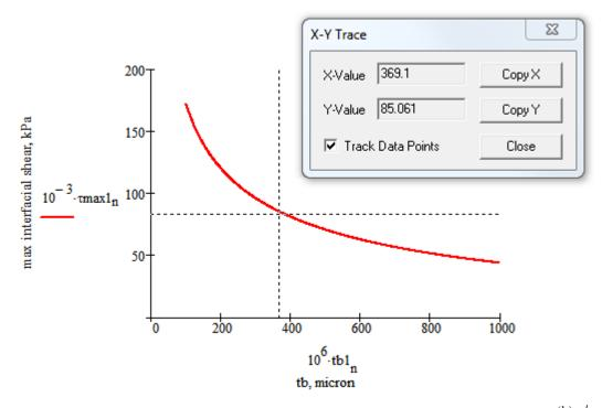
The target shear stress value is half of the value found in item (b) above, i.e.,  $\tau_{\text{max}}^{(b)}/2 \approx 85$  kPa. As shown in the above plot, the approximate value of  $t_b$  that will give a shear stress of approximately 185 kPa is  $t_{b1} = 369 \text{ }\mu\text{m}$ . If more accuracy is needed, then, by iterations, we find that  $t_{b1} = 360 \text{ }\mu\text{m}$  gives  $\tau_{\text{max}}(t_{b1}) = 86.3$  kPa, which exactly half of the one found in item (b) above.
