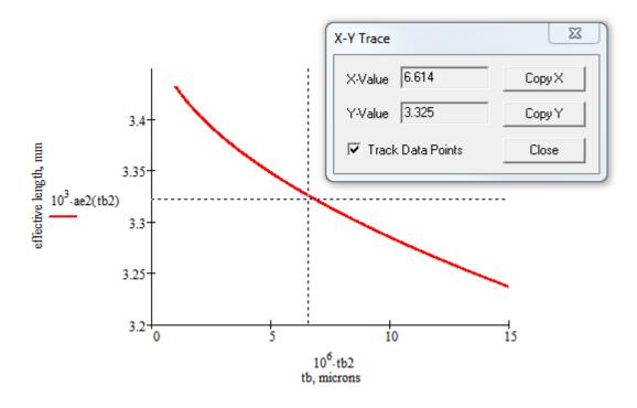
The approximate value is  $t_{b2} \approx 6.6 \,\mu\text{m}$ . This value should be accurate enough for practical purposes because adhesive thickness is not easy to control very precisely.
