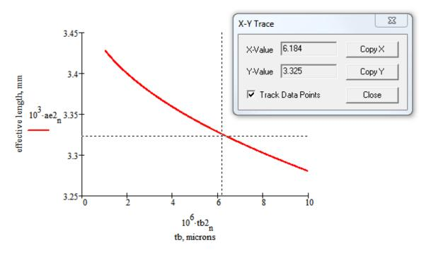
The approximate value is  $t_{b2} \simeq 6.2 \ \mu\text{m}$ . This value should be accurate enough for practical purposes because adhesive thickness is not easy to control very precisely.
