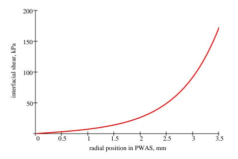
(b) The maximum shear stress is found at the PWAS edge, i.e., r=a; its value is
