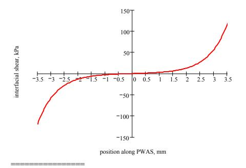
(b) The maximum shear stress is obtained at the ends of the PWAS, i.e., at  $x = \pm a = \pm 3.5$  mm
