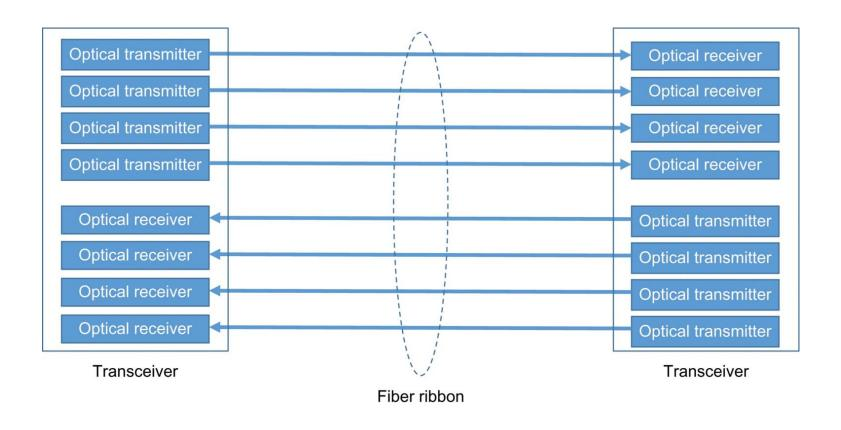
Figure A1.2: A parallel optical link illustrating four transmit and receive lanes.
