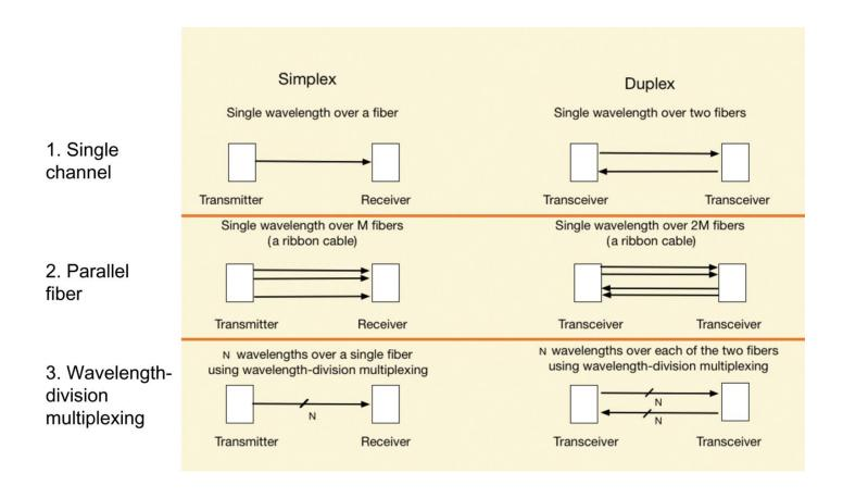
Figure A1.1: The main three approaches used for optical communications.
