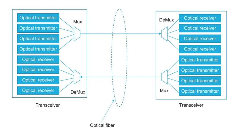
**Figure A1.3:** A CWDM4 transceiver optical link using wavelength-division multiplexing.
