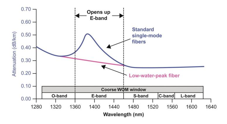
Figure A1.4: Optical attenuation curve of a germanosilicate fiber.
