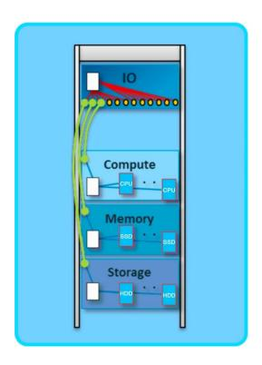
**Figure 1.4:** Disaggregated server where compute, storage, and memory are each pooled and they share networking. Max Smolaks, "Ericsson to sell Intel's hyperscale kit to network operators", ,http://www.datacenterdynamics.com/content-tracks/servers-storage/ericsson-to-sell-intels-hyperscale-kit-to-network-operators/93484.fullarticle., March 3, 2015.
