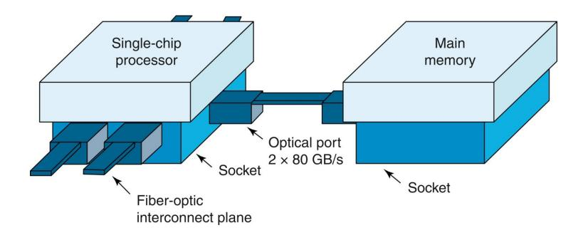
**Figure 1.3:** Optics to interconnect chips. r 2016 IEEE. Reprinted, with permission, from Levi AFJ. Challenges for photonics in future systems. In: Biophotonics/optical interconnects and VLSI photonics/WBM microcavities, 2004 Digest of the LEOS summer topical meetings; 2004. p. 12. ttp://dx.doi.org/10.1109/LEOSST.2004.1338675
