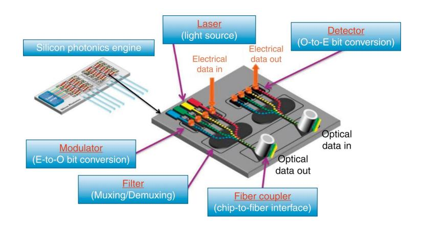
**Figure 1.2:** Silicon as an optical integration platform. Julien Happich, "CMOS-compatible intra-chip photonics brings new class of sensors", ,http://www.analog-eetimes.com/news/cmos-compatible-intra-chip-photonicsbrings-new-class-sensors., Courtesy of EETimes, October 15, 2013.
