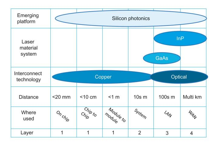
**Figure 1.1:** The reach of silicon photonics and other interconnect technologies. Based on "On-board Optical Interconnect," CTR III TWG Report #3, MIT Microphotonics Center, April 2013, figure 2.
