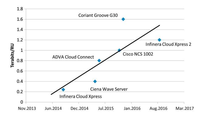
**Figure 5.6:** Data center interconnect introduction dates and per-rack-unit capacity.
