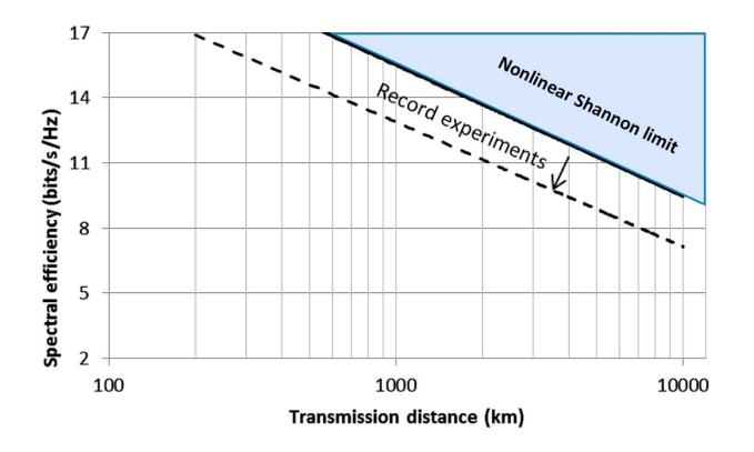
**Figure 5.3:** How the nonlinear Shannon limit of fiber varies with distance. Based on information from Bell Labs.
