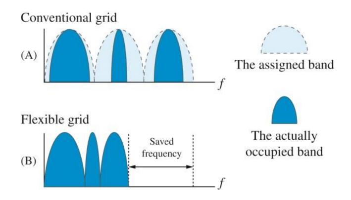
**Figure 5.7:** (A) Conventional and (B) flexible grid illustrated. Japanese Journal of Applied Physics.
