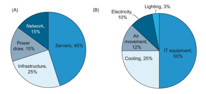
**Figure 6.7:** Typical data center costs and energy consumption breakdowns. (A) Data center costs and (B) data center energy consumption. (A) Data from Microsoft (B) Data from Computerworld from EYP Mission Critical Facilities Inc, New York.
