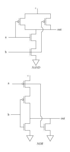
FIGURE D.1: Two-input NAND and NOR complementary logic gates..
