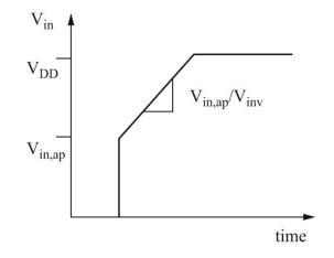
FIGURE D.2:: SakuraieNewton model for gate input voltage.
