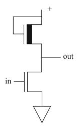
FIGURE D.2:: An nMOS inverter..
