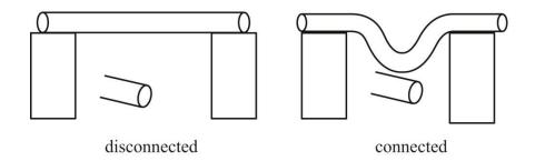
Figure 7.2: A switched connection built from a suspended nanotube.
