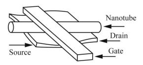
Figure 7.1: A nanotube transistor.
