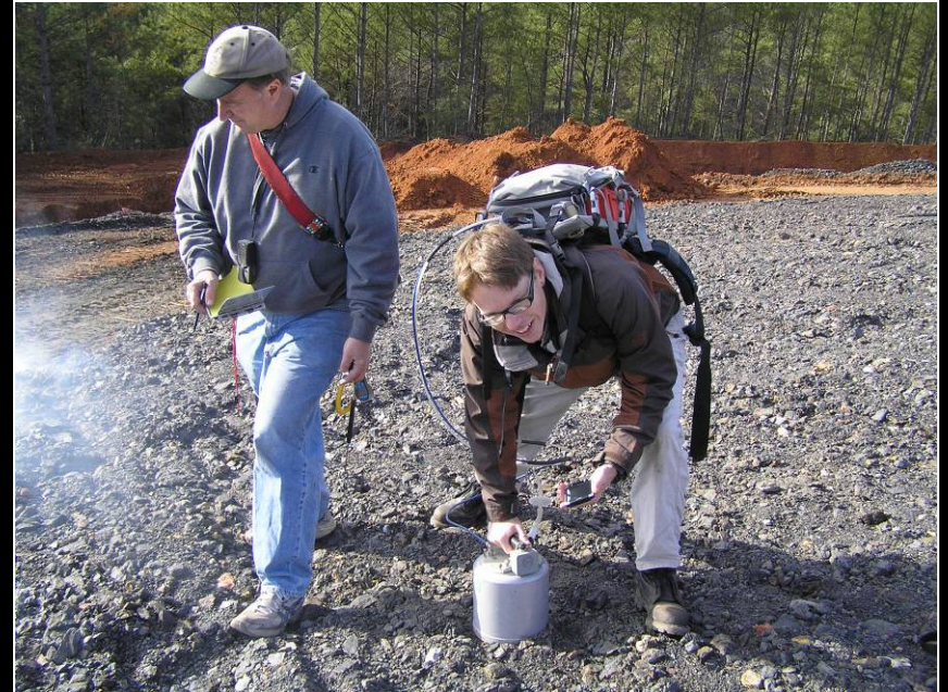
Application of the CO 2 accumulation chamber at the Mulga Gob Fire. Photo by Glenn Stracher.
