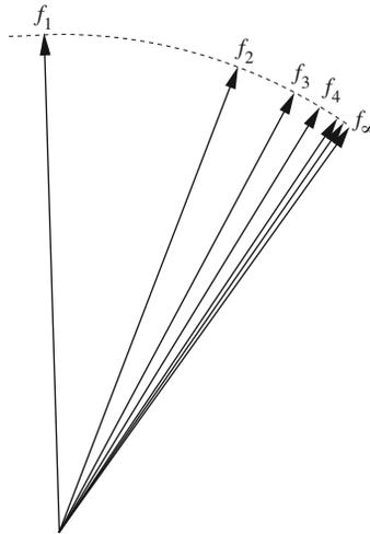
**Fig. B.1.** A pictorial representation of the Hilbert space. We have a vector space (each vector represents a wave function) and a series of unit vectors  $f_i$ , that differ less and less (Cauchy series). If any convergent Cauchy series has its limit belonging to the vector space, then the space represents the *Hilbert space*.
