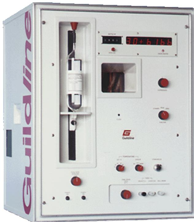
**FIGURE S16.21** Autosal inductive salinometer in common use in laboratories for salinity analyses. Source: From Guildline (2009).
