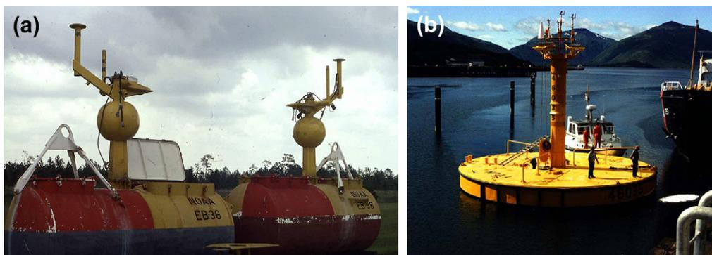
**FIGURE S16.40** (a) Bumble bee buoys used in the North Pacific. (Photo courtesy of W. Emery.) (b) 12 meter disc buoy. Source: From NOAA NDBC (2008).
