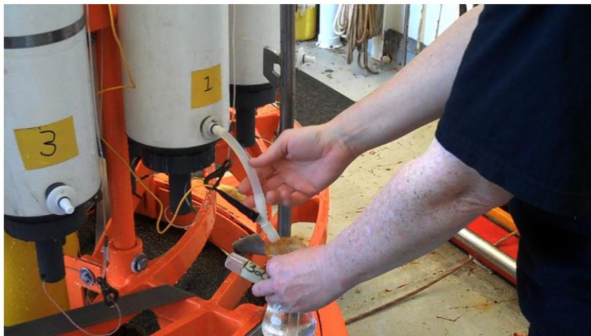
FIGURE S16.22 Drawing an  $\text{O}_2$  sample from a Niskin bottle. (Photo courtesy of J. Swift.)
