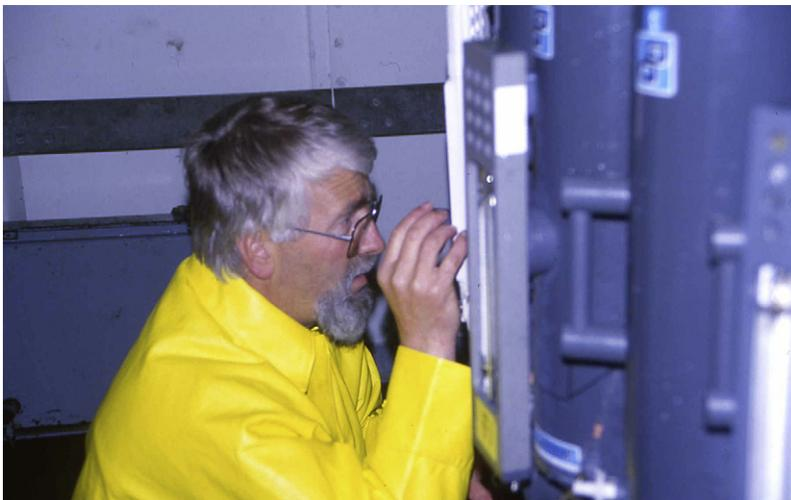
**FIGURE S16.14** Reading reversing thermometers. (Photo courtesy of W. Emery.)
