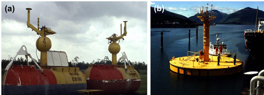
**FIGURE S16.40** (a) Bumble bee buoys used in the North Pacific. (Photo courtesy of W. Emery.) (b) 12 meter discus buoy. Source: From NOAA NDBC (2008).
