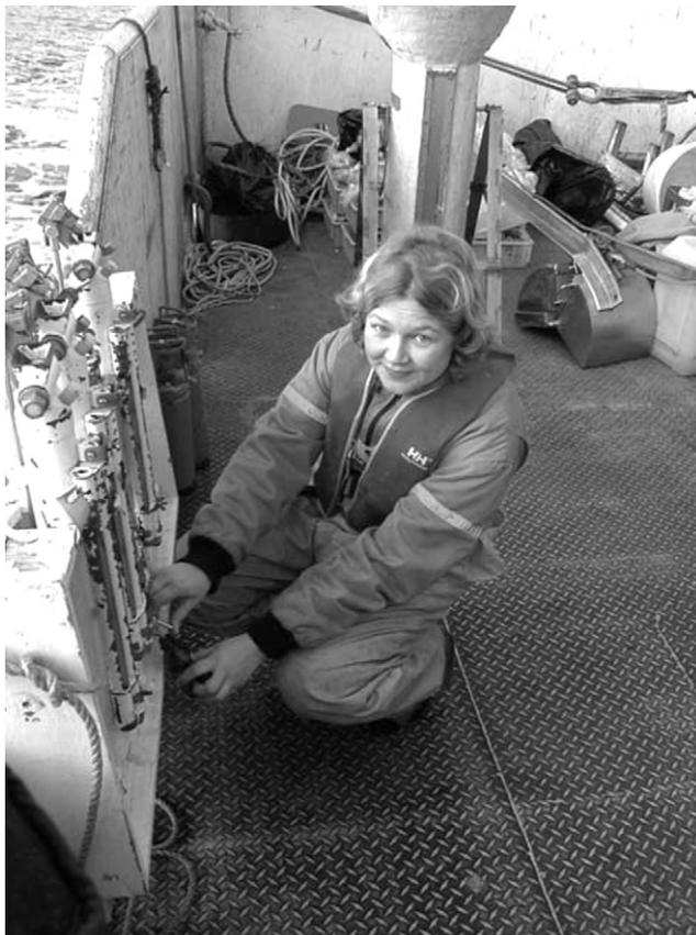
FIGURE S16.20 Drawing a salinity sample from a Nansen bottle. (Photo courtesy of W. Emery.)
