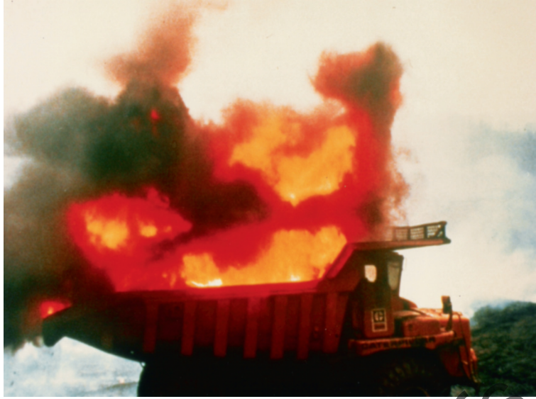
Figure 1.2.4. Combustion enhanced by excavating hot coal in the presence of an unlimited supply of oxygen. Photo courtesy of the West Virginia Department of Natural Resources.
