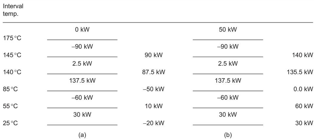
From (b) pinch occurs at interval temperature 85°C.
