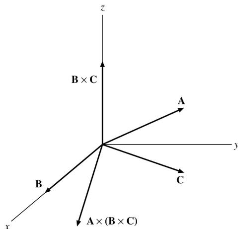
FIGURE 1.17  $\mathbf{B}$  and  $\mathbf{C}$  are in the  $xy$ -plane.  $\mathbf{B} \times \mathbf{C}$  is perpendicular to the  $xy$ -plane and is shown here along the  $z$ -axis. Then  $\mathbf{A} \times (\mathbf{B} \times \mathbf{C})$  is perpendicular to the  $z$ -axis and therefore is back in the  $xy$ -plane.
