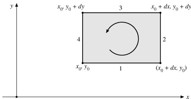
FIGURE 1.24 Circulation around a differential loop.
