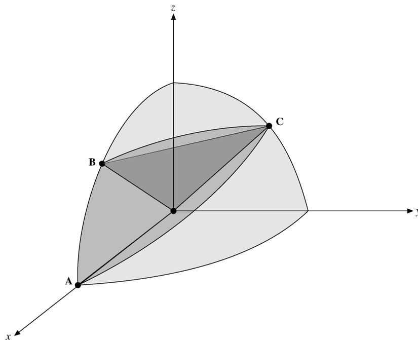
FIGURE 1.14 Spherical triangle.
