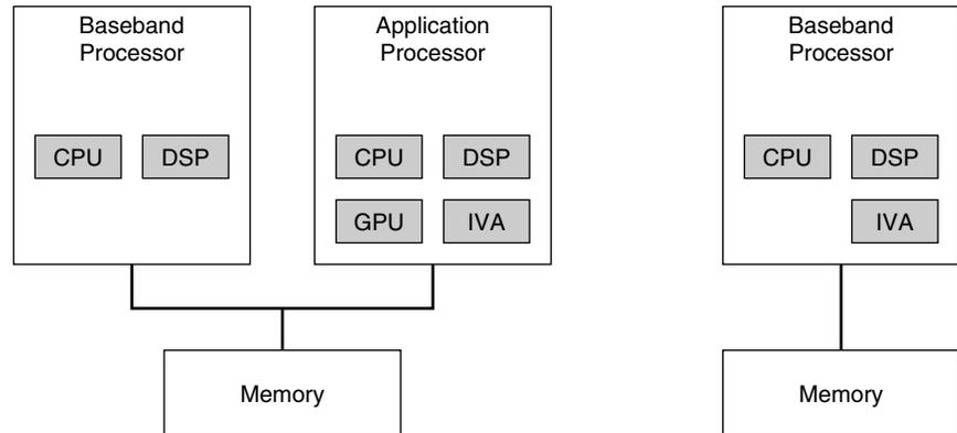
**Figure 1.3:** System architecture of a typical high-end smart phone (*left*) and a feature phone (*right*) in late 2007. Note that feature phones often include an Imaging and Video Accelerator (IVA), whereas a Graphics Processing Unit (GPU) is still relatively uncommon even in the smart phone segment.
