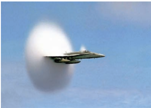
FIGURE 1.8. A photograph of the sound barrier being broken by a US Navy jet as it crosses the Pacific Ocean at the speed of sound just 75 feet above the ocean. Condensation of water is caused by the rapid expansion and subsequent adiabatic cooling of air parcels induced by the shock (expansion/compression) waves caused by the plane outrunning the sound waves in front of it. Photograph was taken by John Gay from the top of an aircraft carrier. The photo won First Prize in the science and technology division of the World Press Photo 2000 contest.
