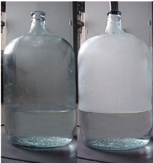
FIGURE 1.6. Warm water is poured into a carboy to a depth of 10 cm or so, as shown on the left. We leave it for a few minutes and throw in a lighted match to provide condensation nuclei. We rapidly reduce the pressure in the bottle by sucking at the top. The adiabatic expansion of the air reduces its temperature and hence the saturated vapor pressure, causing the vapor to condense and form water droplets, as shown on the right.
