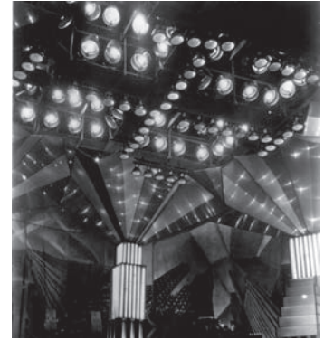
FIGURE 1.3 Early tungsten units in use on the set of Broadway . The dome-shaped units were called “rifles” for their ability to project light at a distance. The open-face units were called “Solar Spots.” Films were “slow” back then (meaning they needed large amounts of light to get a good exposure). Lenses were also slow; the result was that sets had to be lit to a very high lighting level. (Photo courtesy of Mole–Richardson Co.)
