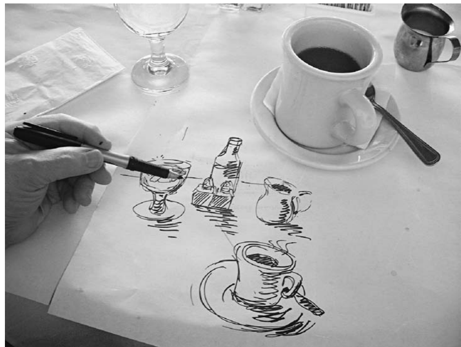
Figure 1-3 Hart's example of a quick concept sketch drawn on a paper tablecloth in a restaurant. Notice the use of basic geometric shapes and shading.
