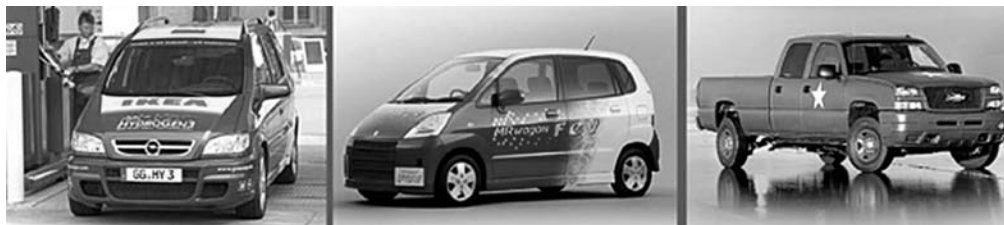
Figure 9.5 The GM HydroGen3 system architecture (60 kW at the wheels) has been scaled down for the integration into a Suzuki MR Wagon FCV (38 kW at the wheels), and scaled up for the propulsion of a Chevrolet Silverado military truck (120 kW at the wheels).
