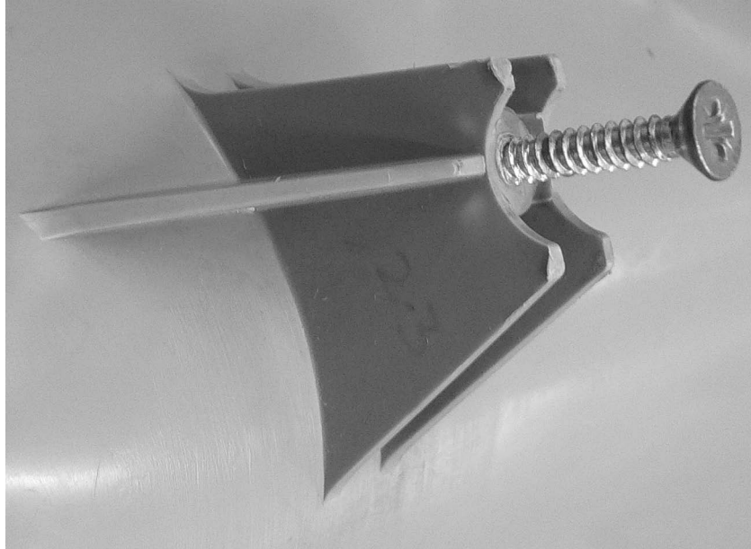
Figure 1.5 Self-tapping screw for attached tubular metal legs, and the boss with buttresses under the seat of a PP stacking chair.
