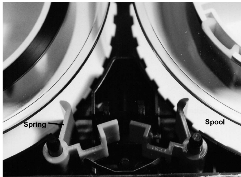
Figure 1.3 Mechanism that locks the spools when the tape is not being played, as seen inside a video cassette.
