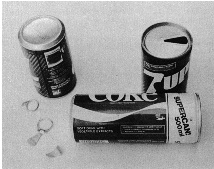
Figure 1.5 The aluminium drink can is an innovative product. The body is made from a single slug of a 3000 series aluminium alloy. The can top is a separate pressing which is fastened to the body by a rolled seam once the can has been filled. There are limits to one-piece construction.
