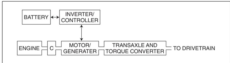
that disconnects the engine from the transaxle when it is switched off for electric propulsion but connects the engine to the transaxle for engine-only power or for combined engine electric motor operation. In other vehicles, the engine and motor are coupled to the drivetrain via a power-splitting device capable of controlling the power split between IC engine and electric motor.
