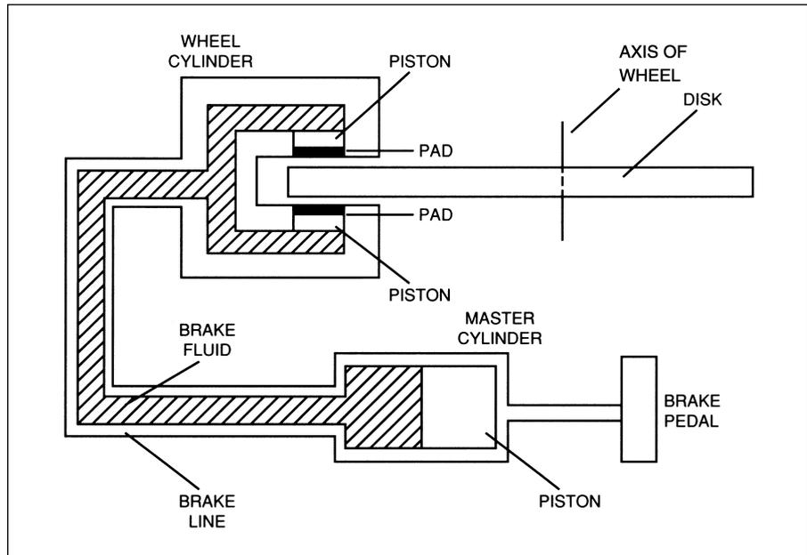
hydraulic pressure is applied through the brake fluid to force the brake pads against the disk. The braking force that decelerates the car results from friction between the disk and the pads.
