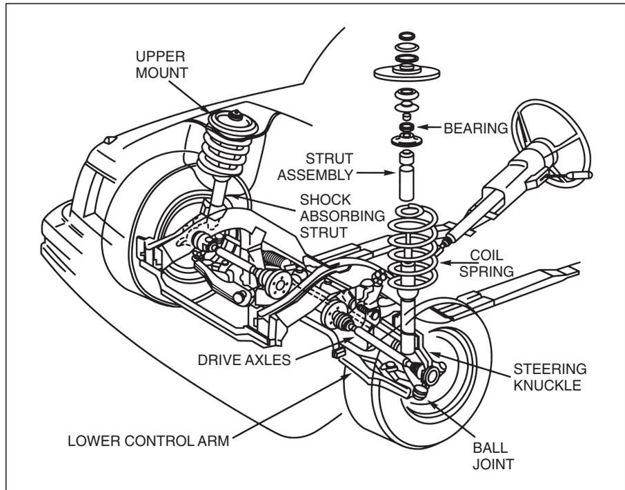
Similar to the springs, the shock absorbers (struts) also produce a force that acts to support the weight of the car. However, unlike the springs, the shock absorbers produce a force in response to the motion of the wheel assembly relative to the car body. Figure 1.16 is an illustration of a typical shock absorber.
