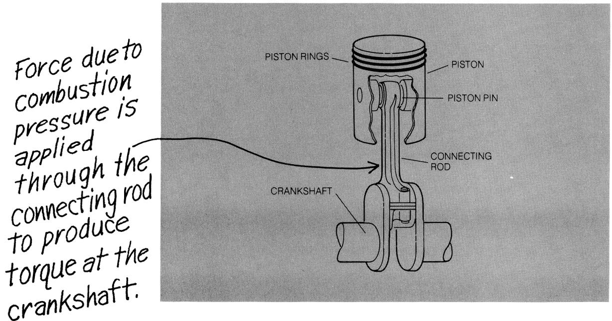
crankshaft by connecting rods, as shown in Figure 1.3. The crankshaft converts the up and down motion of the pistons to the rotary motion and the torque needed to drive the wheels.
