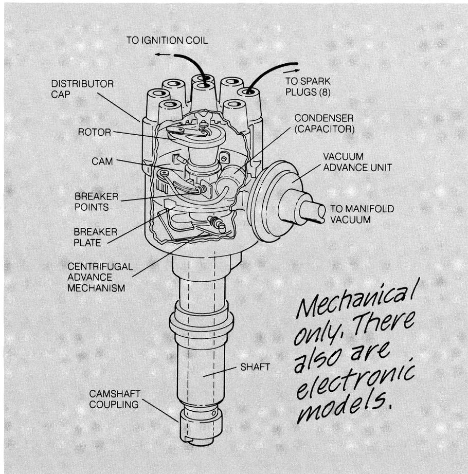
engine, the breaker points have been replaced with an electronic control module in which a power transistor controls the coil current as explained in Chapter 5.
