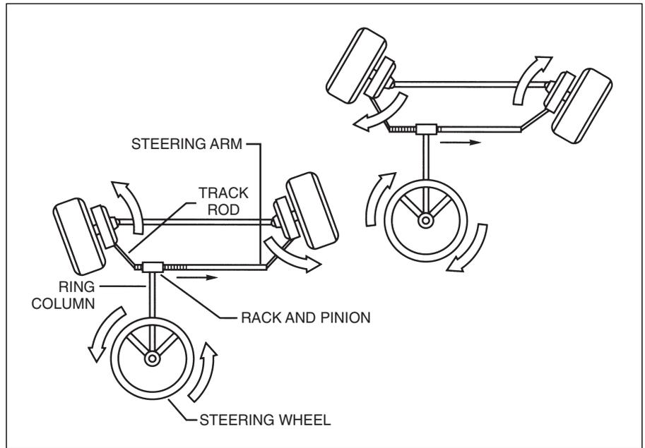
the vehicle weight for any given steering angle, considerable driver effort is required for large cars, particularly at low speeds and when parking.
