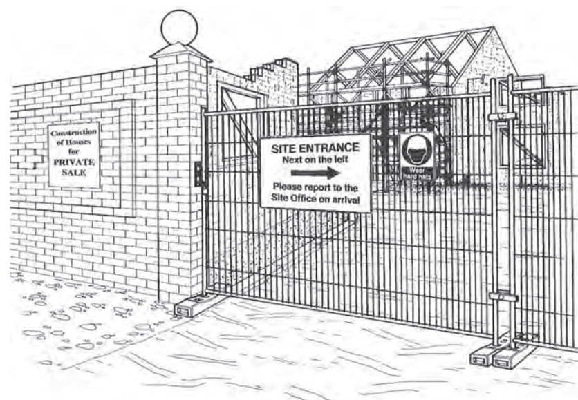
Figure 16.1 Secure site access gate.
