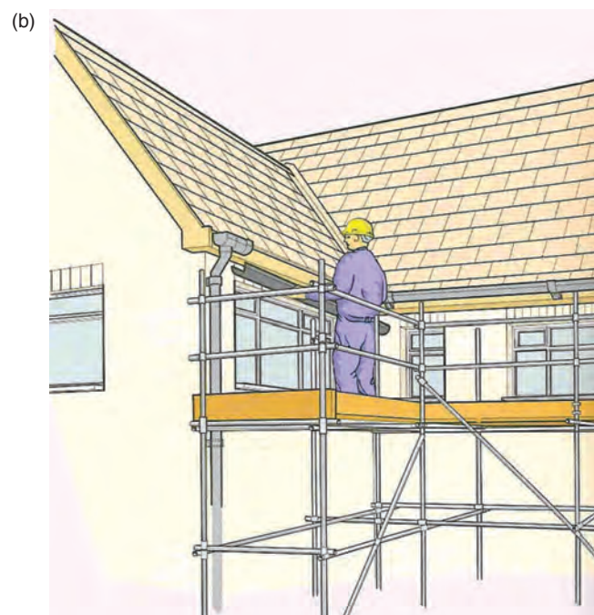
Figure 16.6 (a) Typical independent tied scaffold. (b) fixed scaffold left in place to fit the gutters.
