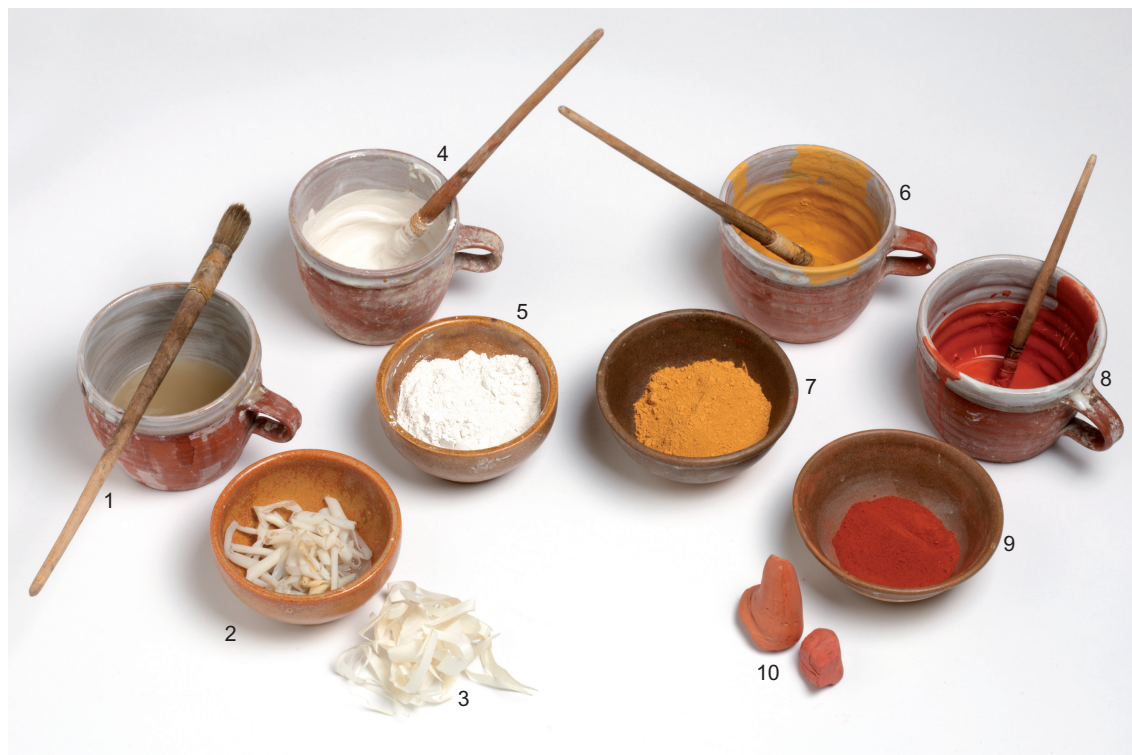
Some gilders' materials: 1. Parchment glue size with a hog hair brush. 2. Wet parchment clippings. 3. Dry parchment clippings. 4. Powdered gypsum in glue size and hog hair brush. 5. Powdered gypsum. 6. Powdered yellow ochre in glue size with hog hair brush. 7. Powdered yellow ochre. 8. Red bole in glue size with squirrel hair mop. 9. Powdered Armenian bole. 10. Cone and lump of bole.
